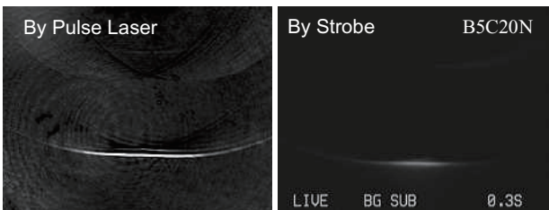
Fig.3 Comparison between the pulse laser system and the conventional stroboscope system
