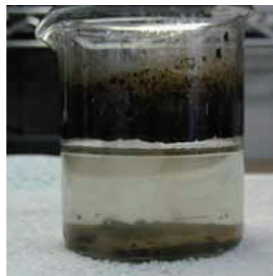
Fig.4 Transparent appearance of the oil sand suspension stood for 24 h following 120 min sonication.
