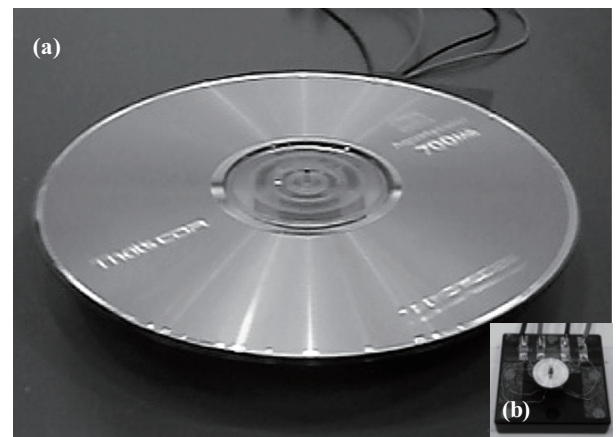
Fig. 6. Overviews of cantilever-type motor and stator with r_v = 4 mm: (a) motor rotor with CD-R shaped rotor, (b) stator vibrator.
