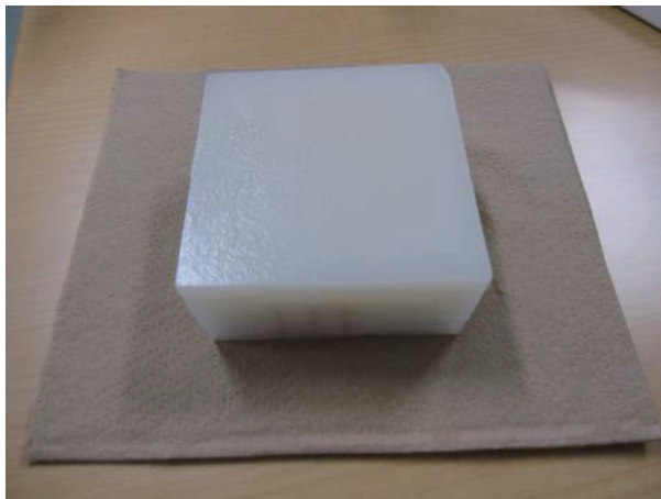
Fig. 2 Calculus phantom used in this study. Three wire targets are embedded in an agar gel.
