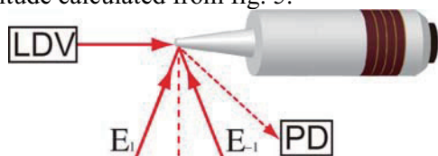
Fig. 4 Measurement set up for the vibration amplitude of bolt-clamped Langevin transducer.
