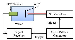
Fig.2 Experimental setup for measuring PA signal
