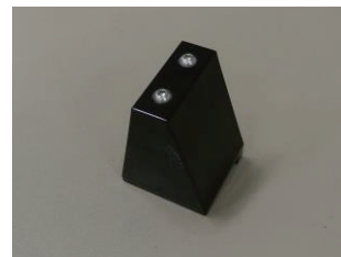
Fig. 2 Used phantom, which is for calibration of Minelyzer.
