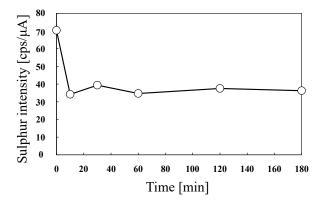
**Fig. 2.** Change of sulphur intensity by NaOH reaction time. ( $H_2O_2$  reaction time: 10 min)
