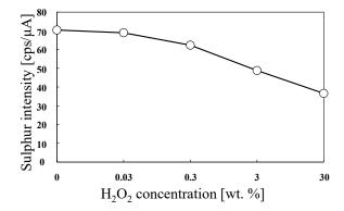
**Fig. 3.** The effect of  $H_2O_2$  concentration on the desulphurization of bitumen
