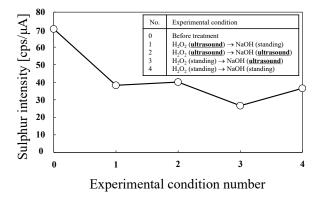
Fig. 4. Sulphur intensity of bitumen after treated with  $H_2O_2$  (30 wt. %) and NaOH with/without ultrasound irradiation
