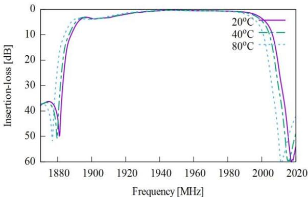
Fig.1 Variation of insertion loss with  $T$ . Solid line: 20°C, solid and dotted line 40°C, and dotted line 80°C.
