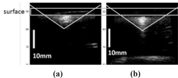
Fig. 6 B-mode images of cavitation bubbles.
