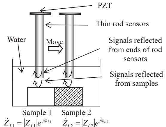
Fig. 1. Phase-contrast imaging procedure.
