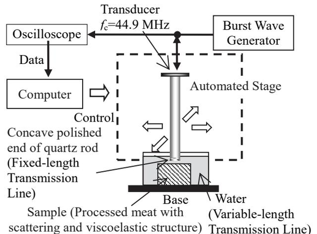
Fig. 3. Schematic diagram of experiment.
