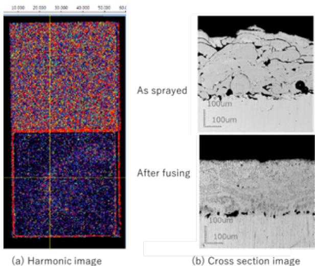
Fig.4 HHI and micrographs of Ni based self-fluxing alloy before and after fusing.
