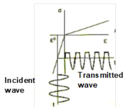
Fig.1 Waveform distortion at closed cracks [4].
