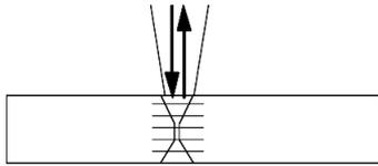
Fig.2 Through-thickness local resonance.
