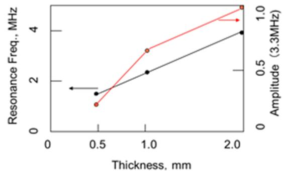
Fig. 6 Change in resonance frequency with thickness.
