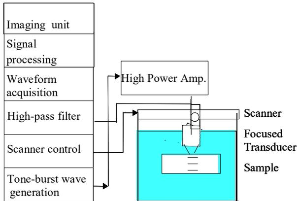
Fig.3 The immersion HHI system.
