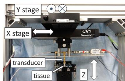
Fig. 1 Overview of self-made scanning acoustic microscopy system in the scanning part.
