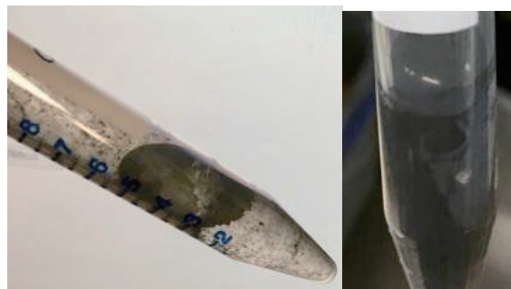
Fig. 1 C65 before (left) and after (right) 1-minute sonication in the ultrasonic cleaner.
