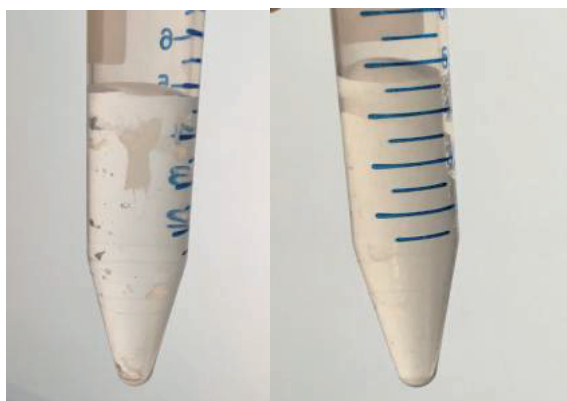
Fig. 2 ZnO before (left) and after (right) 1-minute sonication in the ultrasonic cleaner.
