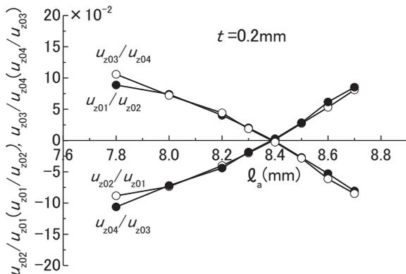
Fig. 3 Analyzed relationships of maximum displacement ratios to short arm length of transverse vibrator.
