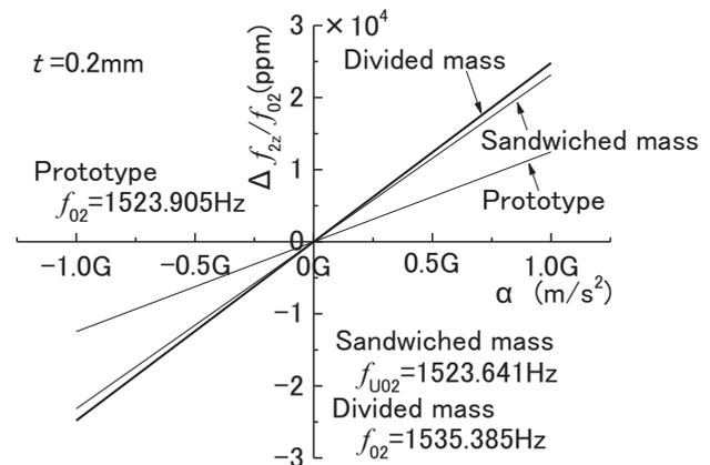
Fig. 5 Comparison of sensor sensitivity.
