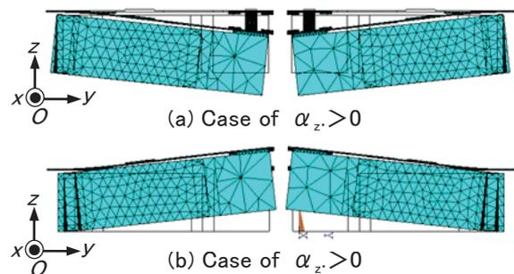
Fig. 2 Movement of mass due to acceleration  $\alpha_z$ .
