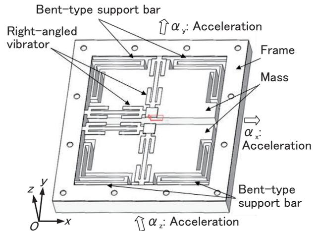
Fig. 1 New structure of three-axis acceleration sensor.
