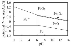
Fig. 4 Potential-pH diagram of Pb.
