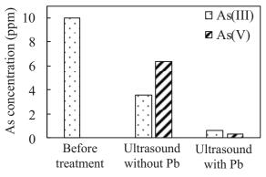
Fig. 3 Residual As(III) and As(V) concentrations before and after treatment using ultrasound with or without Pb electrode which is applied potential of -0.7 V vs. Ag/Ag/Cl.
