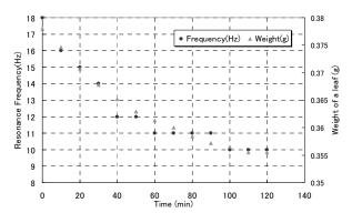
**Fig. 3.** The temporal change of the resonance frequency and the weight of a leaf. gray triangle: the temporal change of a leaf weight, black circle: temporal change of the resonance frequency.
