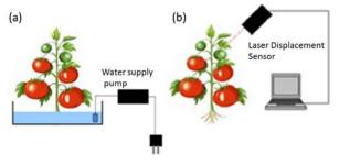
**Fig. 5.** Experimental setup for pseudo water stress to a plant. (a) Before the measurement: a tomato was raised by hydroponic culture, (b) On the measurement: water stress was given by cut the water supply off. The resonance frequency of a leaf was measured by a laser displacement sensor.
