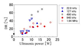
Fig.3 Effect of ultrasonic frequency on relationship between ultrasonic power and DR with Pluronic F-108.
