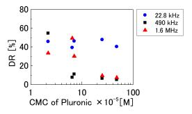
Fig.3 Effect of molecule structure of Pluronic on stability of Pluronic micelle.
