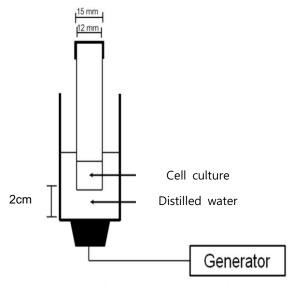
Figure 1 – Experiment setup of the ultrasonic irradiation system.
