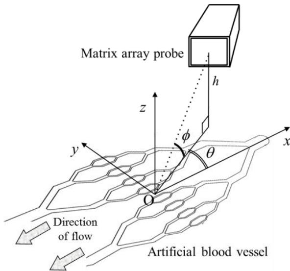
Figure 2: Experimental conditions: probe and capillary relative positions.
