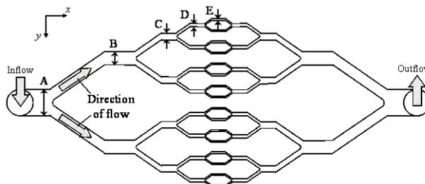
Figure 1: Construction of the multi-bifurcation artificial blood vessel (capillary model).
