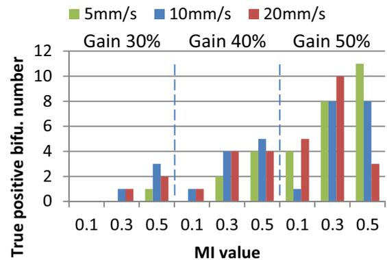
Figure 4: Amount of true positive detected bifurcations depending on flow velocity, echography gain and MI value.
