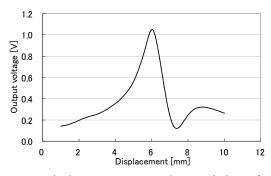
Fig. 5 Displacement-output characteristics of the sensor unit.
