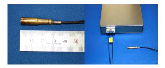
Fig. 4 Newly developed optical vibration sensor system for underwater use.
