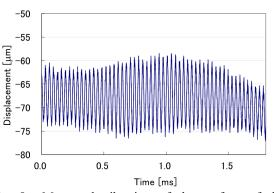
Fig. 8 Measured vibration of the surface of the ultrasonic cleaner.
