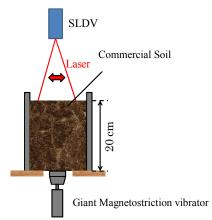
Fig. 2. Experimental setup for propagation velocity.
