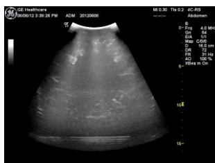
Fig. 3 B-mode image of acoustic cavitation generated in the standing wave acoustic field in water vessel of 150 kHz sonoreactor (B-mode
