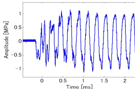
Fig. 3 Time waveform of intense focused ultrasound
