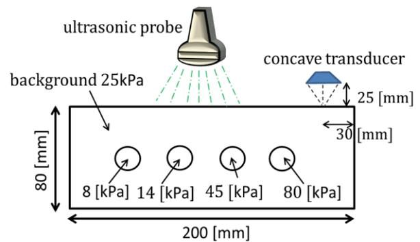
Fig. 1 Experiment configuration to generate and measure shear wave displacement
