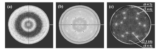
Fig. 2 Pole figures of (a)  $Ta_2O_5/SiO_2$ , (b)  $Ta_2O_5/c-Al_2O_3$  (no pretreatment), and (c)  $c-Al_2O_3$ .
