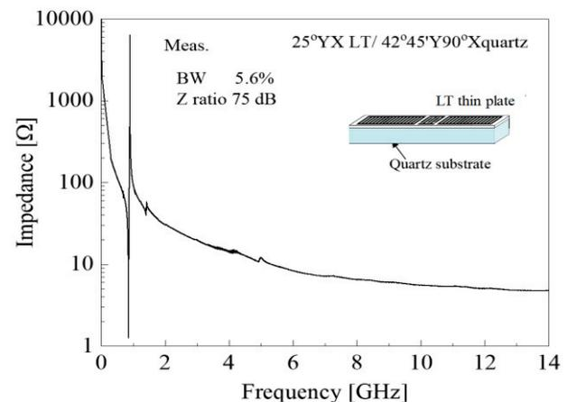
Fig. 1 Measured wide frequency characteristic of HAL SAW resonator composed of 25°YX LT plate bonded 42°45'Y90°X quartz substrate.
