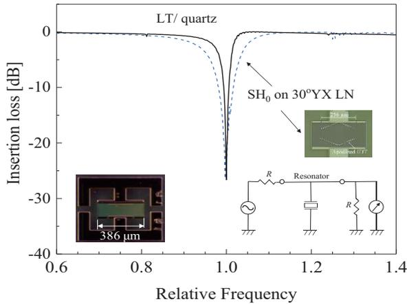
Fig. 2 Measured frequency characteristics of parallel type rejection filters. Solid line: HAL SAW based, Blue broken line: SH<sub>0</sub> based.
