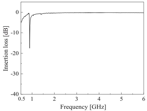
Fig. 5 Measured wide frequency characteristic of series type HAL SAW rejection filter.
