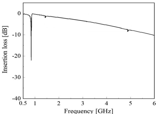
Fig. 4 Measured wide frequency characteristic of parallel type HAL SAW rejection filter.
