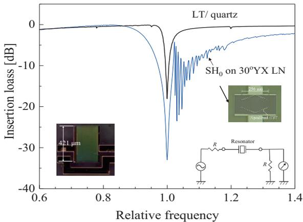
Fig. 3 Measured frequency characteristics of series type rejection filters. Solid line: HAL SAW based, Blue broken line: SH<sub>0</sub> based.
