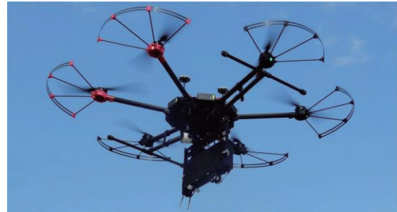
Fig.1. Sound source mounted type UAV in flight.
