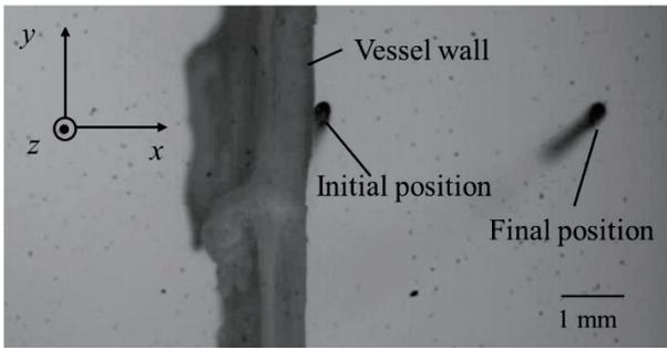
Fig.2 Catheter bending observed by high-speed camera
