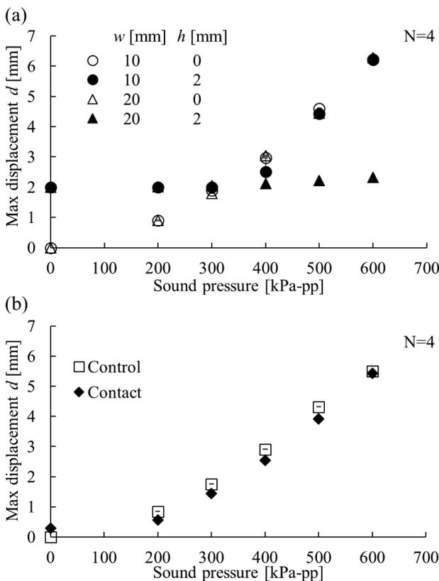
Fig.3 Catheter bending displacement during vessel wall contact ((a) the latex membrane, (b) the rat abdominal aorta)
