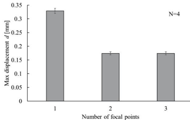
Fig.4 Catheter bending displacement during adhesion of the latex membrane at each focal number
