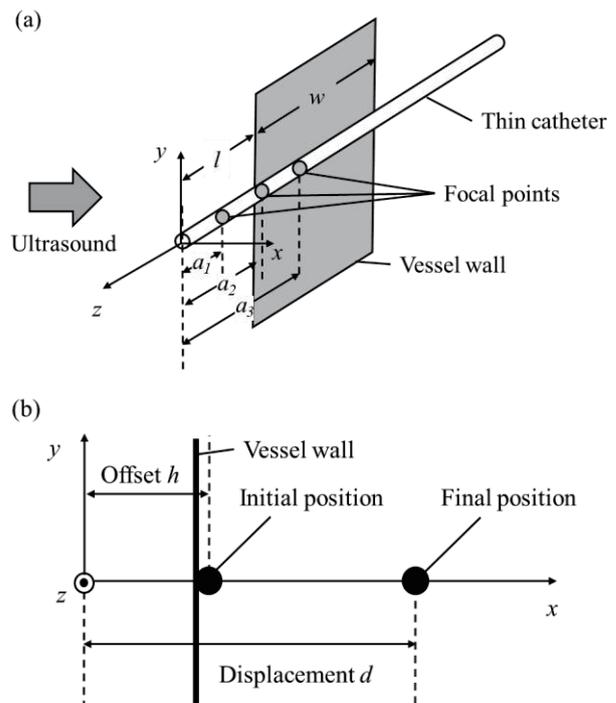
Fig.1 Experiment of the effect of vessel wall contact on catheter bending
