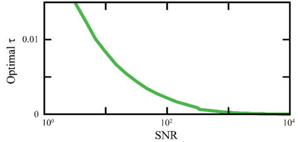
Fig. 3 Relationship between SNR and optimal  $\tau$ .
