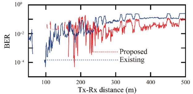
Fig. 5 Relationship between Tx-Rx distance and BER.
