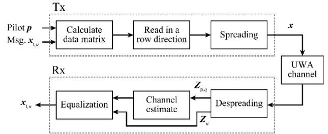
Fig. 1 Block diagram of D-OSDM in Tx and Rx.
